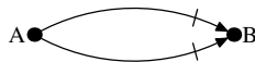
Fig. 5. The gadget for equations of the form x + y = 1 . There is a Hamiltonian path from A to B only if one of the ticked edges is traversed.
